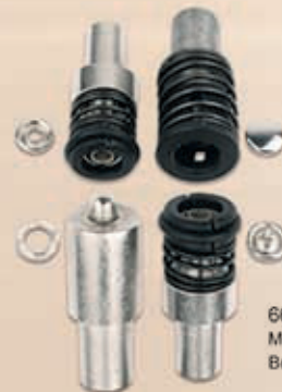
6616-0032 Mould & Dies for Snap Ring Button with Polyester-face
